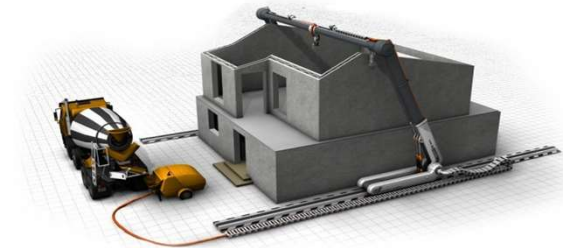
Figure 2: Schematic of a 3D printer and the printed construction [3].
