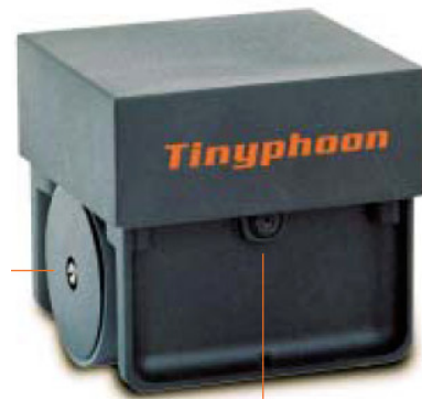
Figure 3-2: Autonomous Robot developed by University of Technology in Vienna [19]
