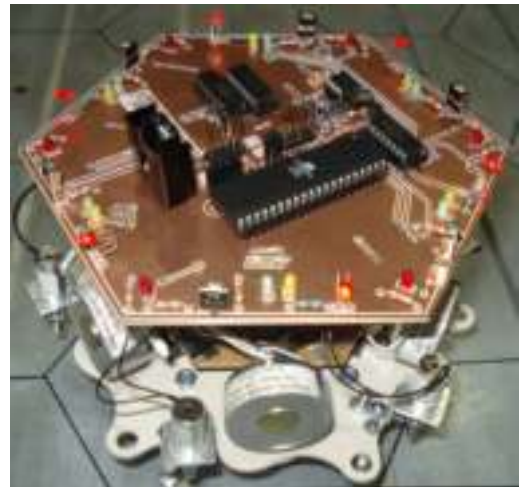
Communication board installed
