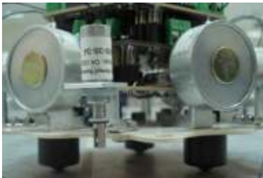
a) Ball transfer units on the module
