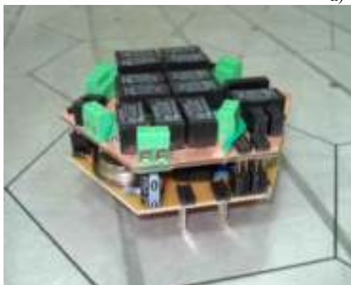
b) Drive circuit installed on the power unit
