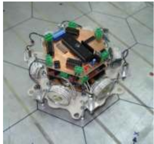
c) Control board installed on the module
