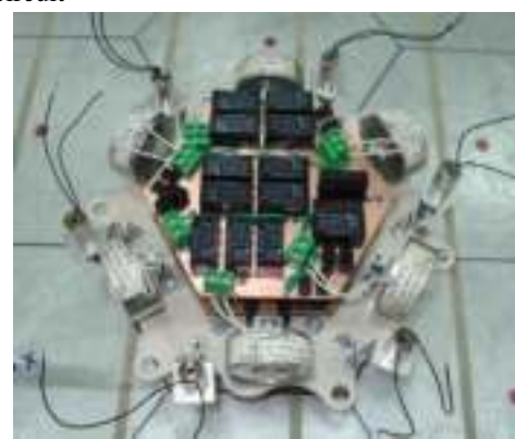
c) Drive circuit installed on the module
