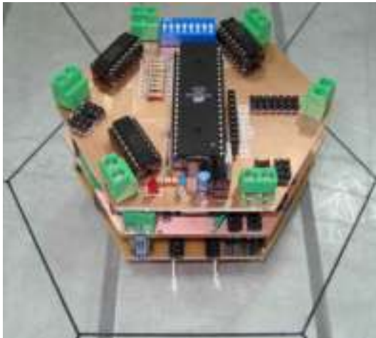
b) Control board installed on drive circuit
