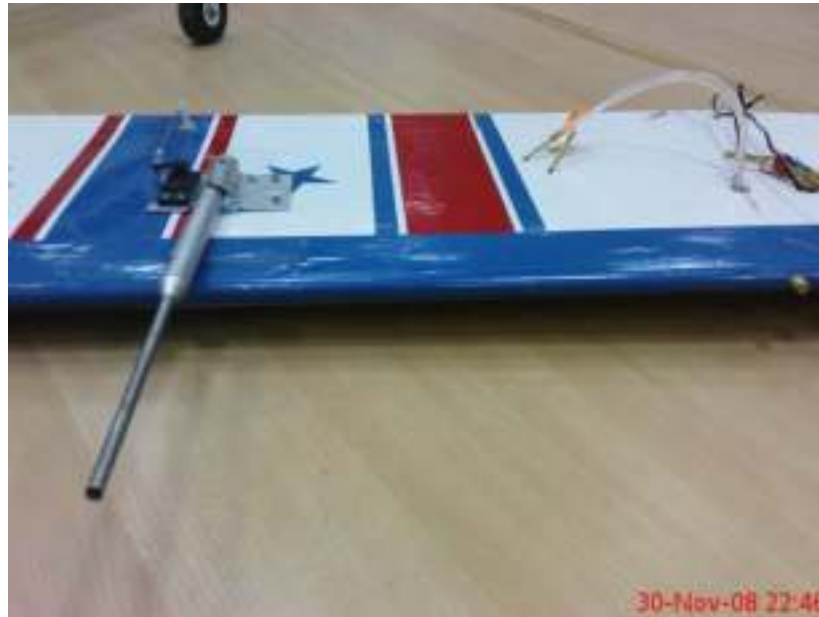
Figure 7.11: Pitot Static Tube Location on the Aircraft
