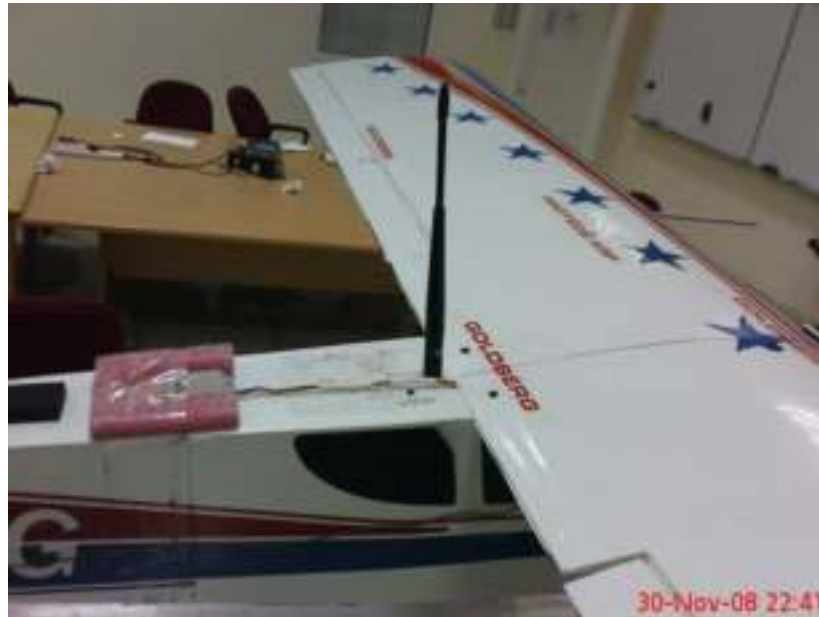
Figure 7.9: RF Antenna Location on the Aircraft
