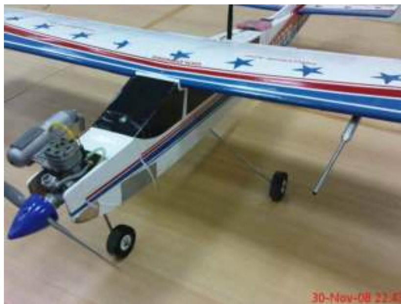
Figure 7.10: Pitot Static Tube Location on the Aircraft
