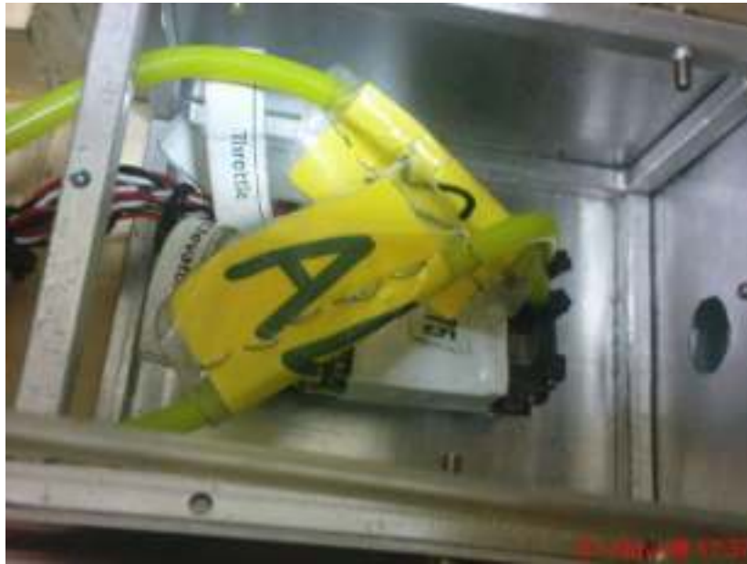
Figure 7.7: Kestrel Autopilot inside the Aluminum box
