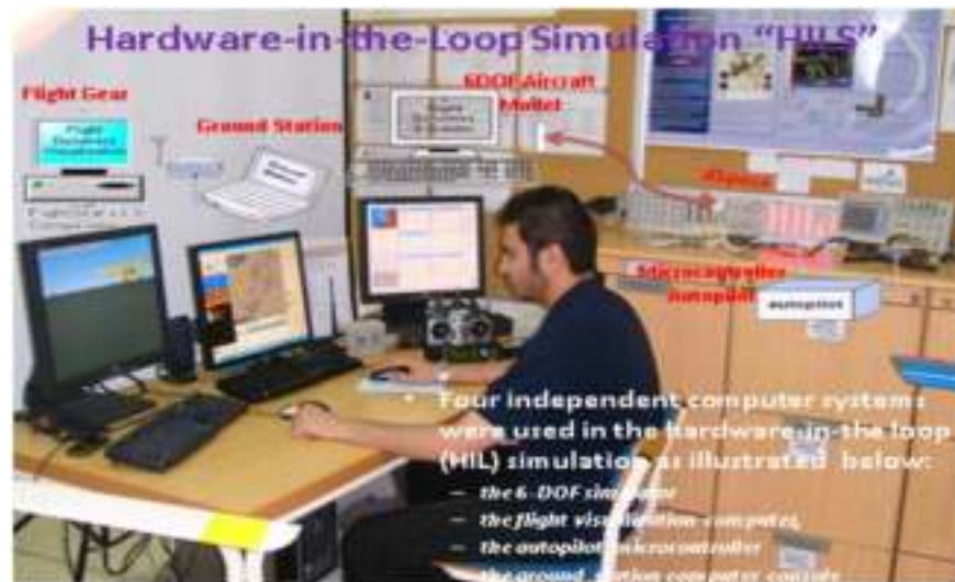
Figure 6.2: Hardware-in-the-loop (HIL) simulation environment
