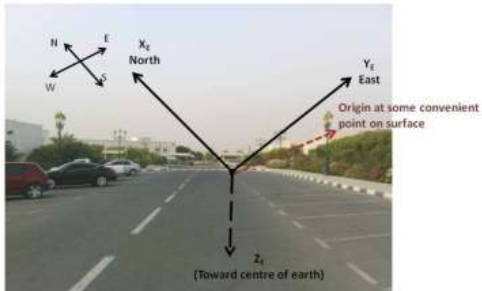
Figure 2.1: Inertial Axis Definition
