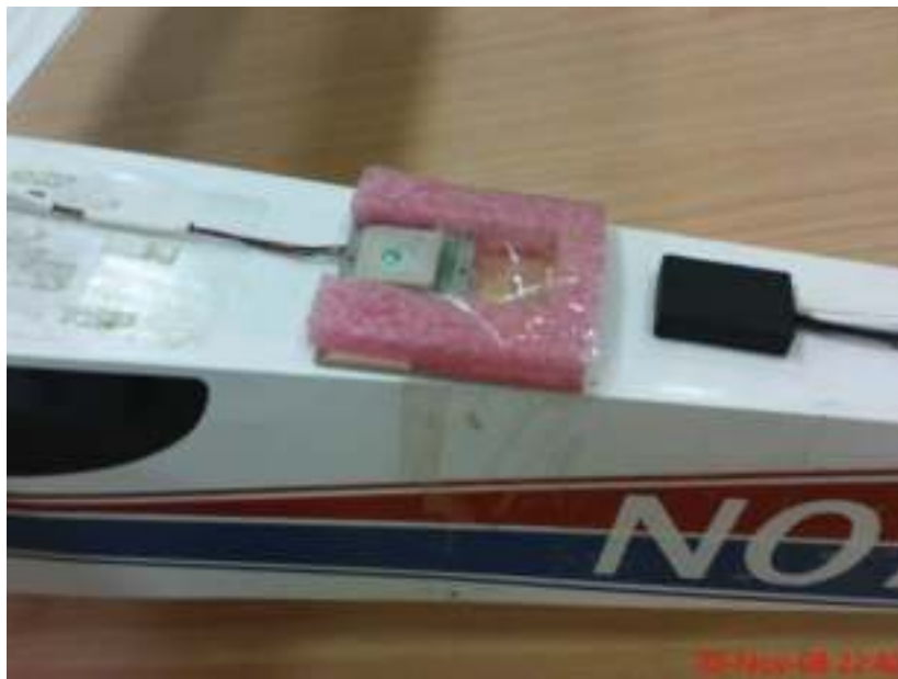
Figure 7.8: GPS Location on the aircraft
