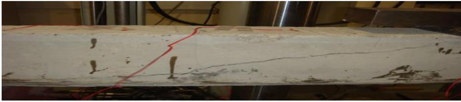
(a) Control beam B1 shear failure
