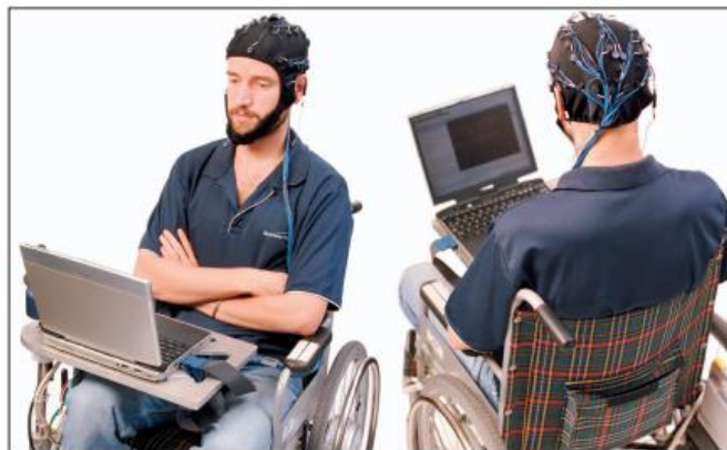
Figure 2.6: A brain-controlled wheelchair acquiring EEG signals via an EEG cap [19].
