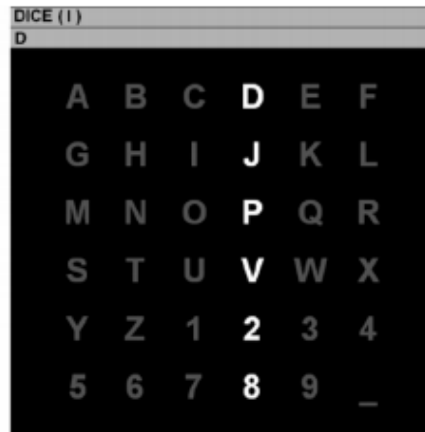
Figure 2.7: A 6 \times 6 matrix for the P300 Event-Related Potential. The rows and columns are highlighted at regular intervals [20].
