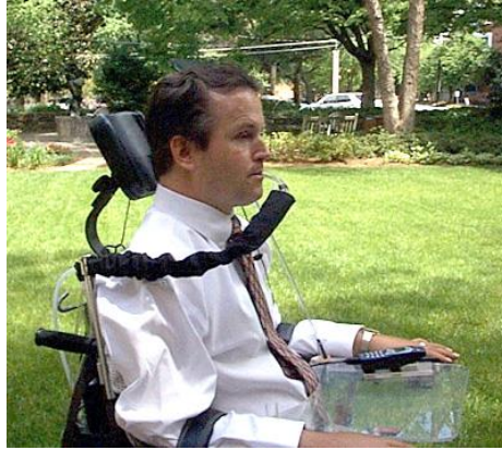
Figure 2.5: Sip-and-Puff Assistive Technology for controlling a wheelchair [18].
