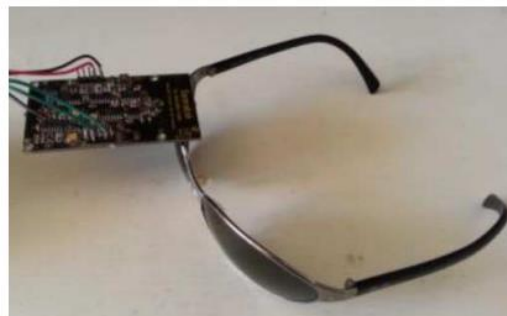
Figure 2.2: A setup using a Doppler sensor to detect eye-blinks [9].
