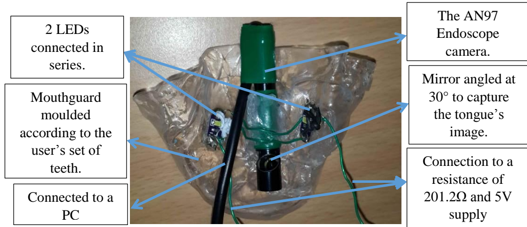
Figure 4.2: The personalized mouthguard along with the LEDs and the Endoscope camera.
