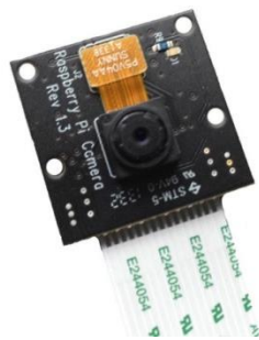
Figure 3.2: Raspberry Pi's NOIR camera along with the board.
