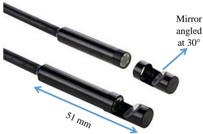
Figure 3.4: The AN97 Endoscope camera along with a 30° mirror added at the camera head.
