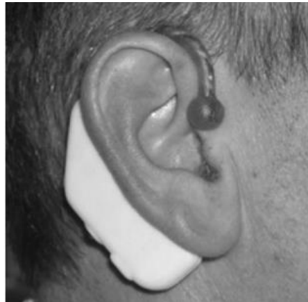
Figure 2.4: A Tooth-click detector device worn behind the ear.
