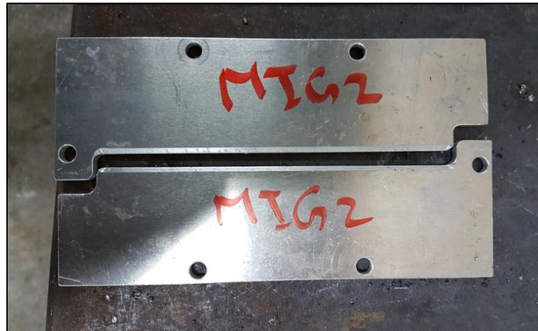
Figure 13: Metallic plates to be welded
