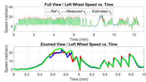
Figure 76: Battery-supercapacitor-fuel cell test, reference, measured, estimated speed of the left wheel.
