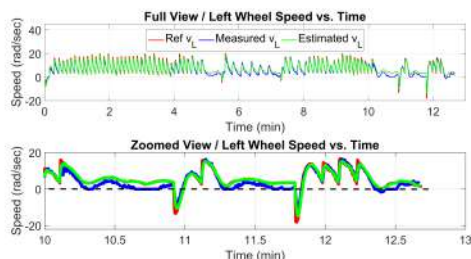
Figure 68: Battery-fuel cell test, reference, measured, estimated speed of the left wheel.
