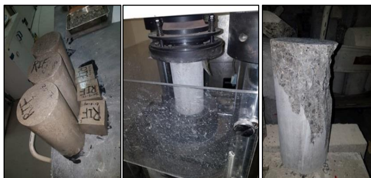
Figure 3-14: Compressive strength testing
