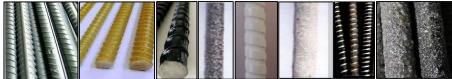
Figure 1-1: From left to right: ribbed steel bars, ribbed AFRP, ribbed CFRP, sand-coated CFRP, grooved GFRP, sand-coated GFRP bars, ribbed BFRP bars, and sand-coated Basalt FRP bars [6, 7, 8].
