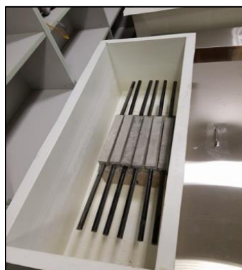
Figure 3-2: Temperature-controlled conditioning tanks
