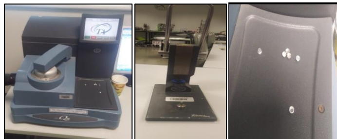
Figure 3-20: DSC apparatus and testing procedures
