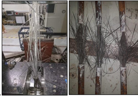
Figure 4-32: Detaching of fibers due to tensile failure
