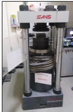
Figure 3-13: Automated compressive strength machine
