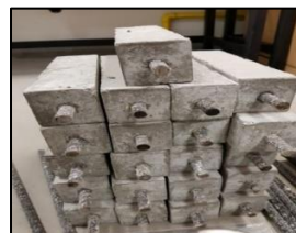
Figure 3-8: Microstructural concrete-wrapped prisms
