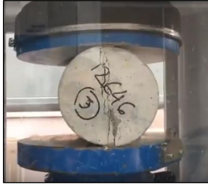
Figure 3-15: Splitting tensile test
