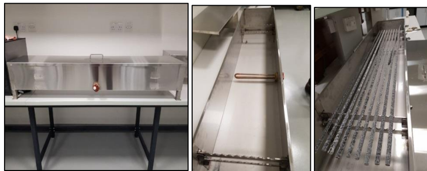
Figure 3-3: Stainless Steel tanks for alkaline conditioning
