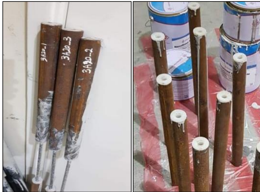
Figure 3-11: Steel grips and teflon rings
