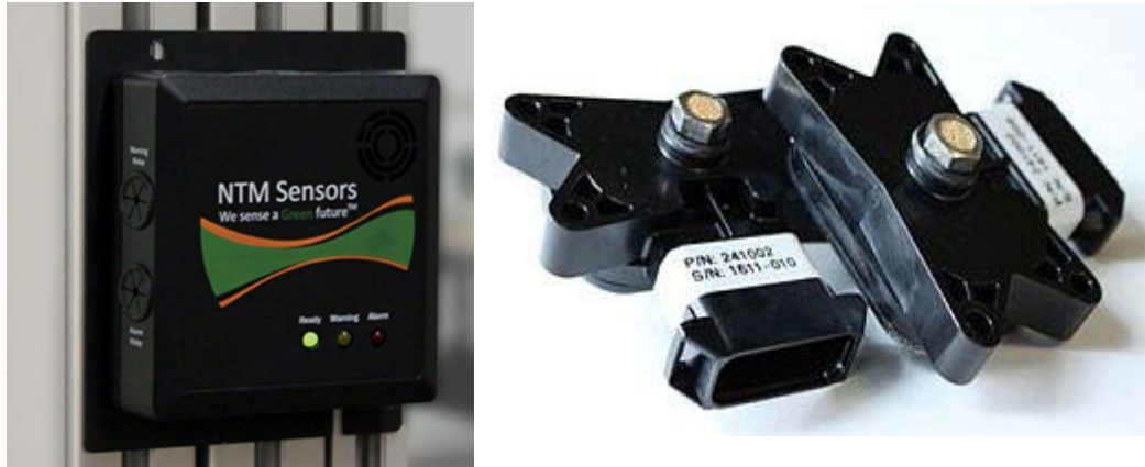
Figure 3.5: NTM hydrogen alarm system [51].
