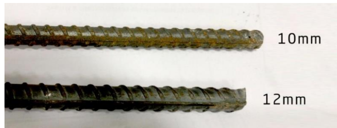
Figure 4: A sample of ribbed steel bars used in this study
