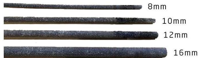
Figure 2: A sample of sand-coated BFRP bars used in this study
