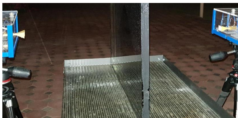
Figure 4.2: Image of one of the penetration loss measurement set up.
