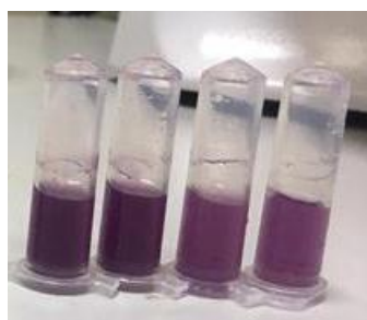
Figure C.3: Attachment confirmation with darker purple color for Immunoliposomes indicating more protein content, after performing BCA assay.
