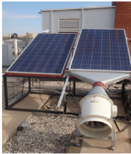
Figure 5. Forced air cooling [19].
