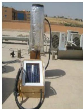
Figure 4. Thermosyphon effect used on PVT system [14].
