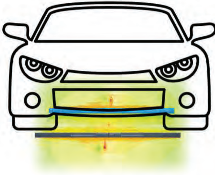
Figure 4.1: Simulation of WPT taking place between the transmitter coil embedded underground, and the receiver coil fixed at the bottom of the car.
