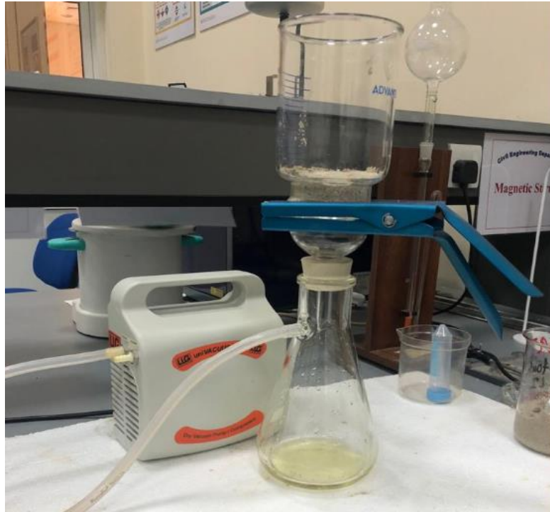
Figure 3.5: Extraction of KI absorbed by the sediments after the density separation
