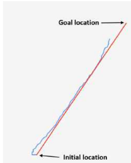
Figure 7: Preliminary testing of navigation module with 2 meters stopping threshold.
