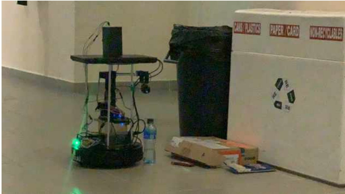
Figure 45: The developed robot before picking up the bottle in indoor Test 2.
