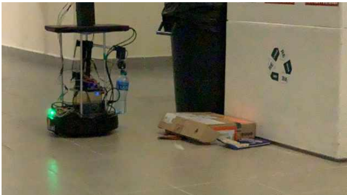
Figure 46: The developed robot picked up the bottle in indoor Test 2.
