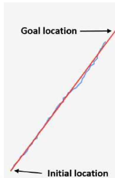
Figure 8: Preliminary testing of navigation module with 1 meter stopping threshold.
