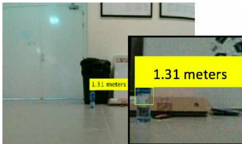
Figure 27: Detected plastic bottle during the indoor test shown in Figure 25.
