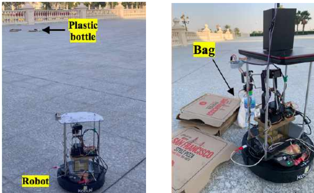
Figure 28: (a) Left: Initial position of the developed robot away from plastic bottle outdoors (b) Right: Final stage of outdoor testing showing successful bottle pickup.
