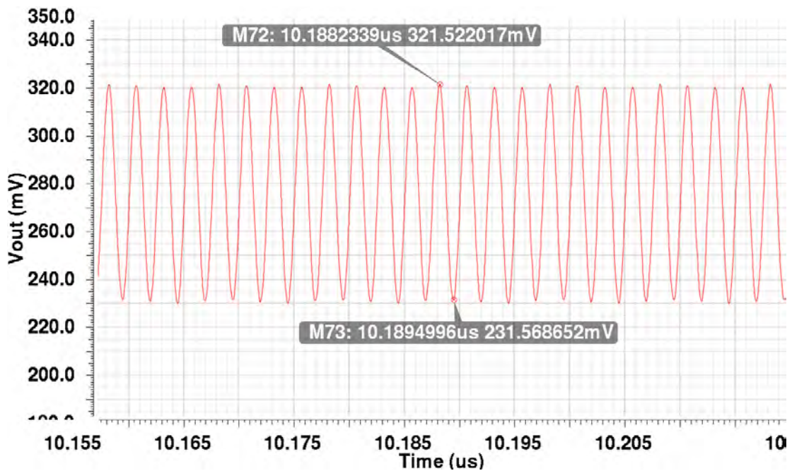
Figure 5.17 LNA total gain = 19.08dBV @400MHz
