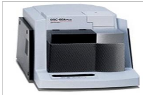
Figure 4.3: Shimadzu DSC-60a Plus Differential Scanning Calorimeter
