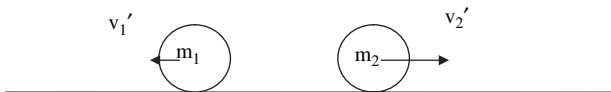
Fig. 2. The figure shows two particles of masses, m_1 and m_2 , and velocities, v_1 and v_2 , after they have collided (1-D collision).
