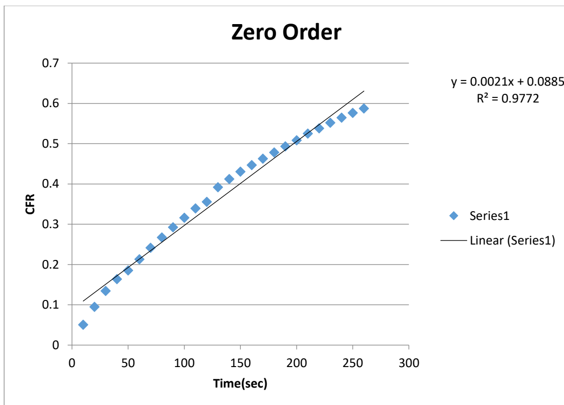
Figure A1: Zero Order Model of the ultra-sound triggered DOX Loaded NH 2 -Fe BDC MOF at a pH level of 7.4 and 37 °C
