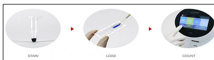
Figure 27: The process of automated cell counting [89]
