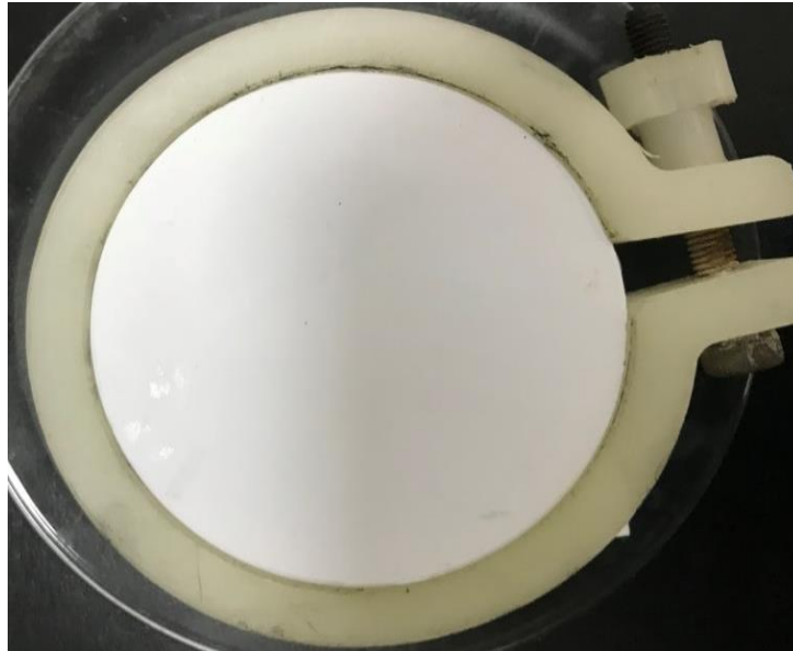
Figure 15: PTFE membrane before adding PANI/IL solution placed on a hoop.
