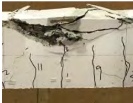
Figure 53: Failure mode of beam 3G16EC.
