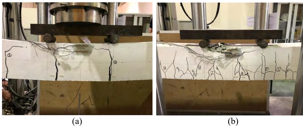
Figure 32: Crack propagation of: (a) 2G8EC; and (b) 2G10UC.
