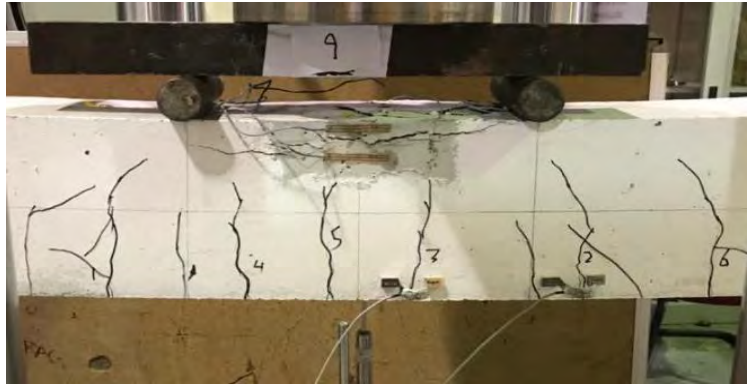
Figure 82 : Cracks propagation of beam 2G26ER.
