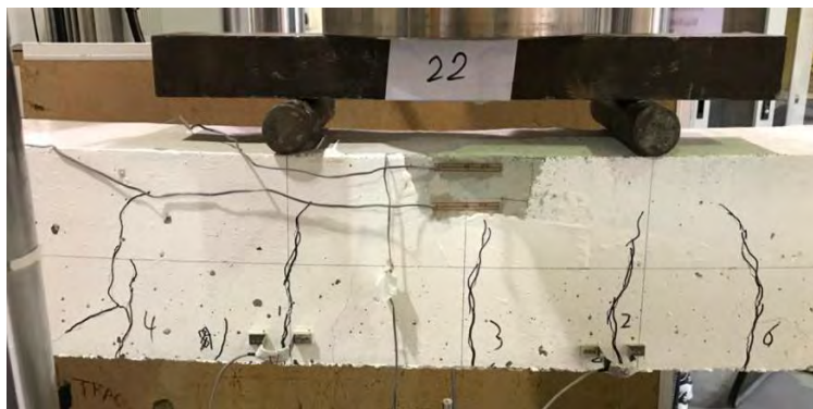
Figure 95: Cracks propagation of beam 2C12EC.
