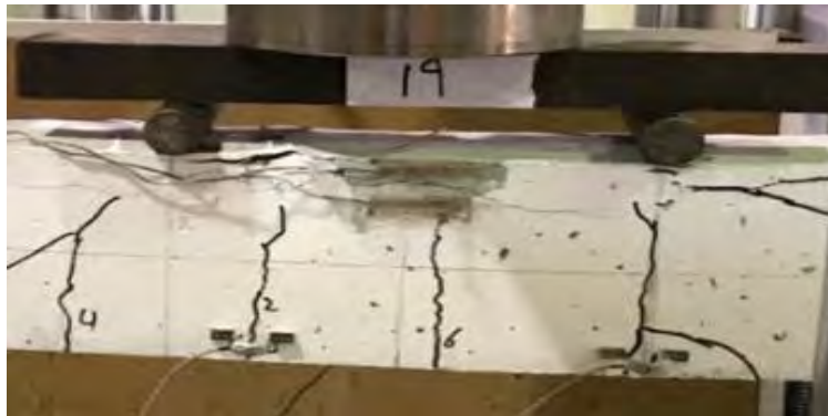
Figure 92: Cracks propagation of beam 2B20EC.
