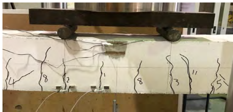
Figure 77: Cracks propagation of beam 2G20EC.
