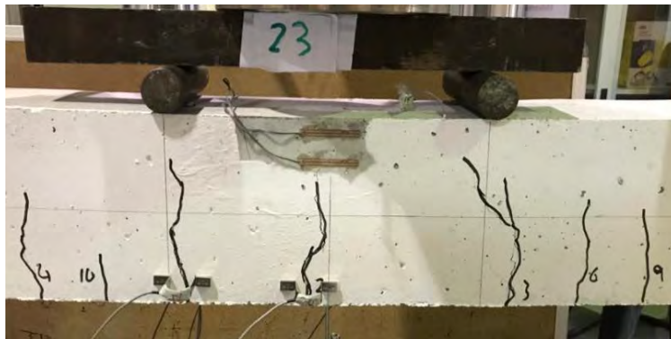
Figure 96: Cracks propagation of beam 2S12.
