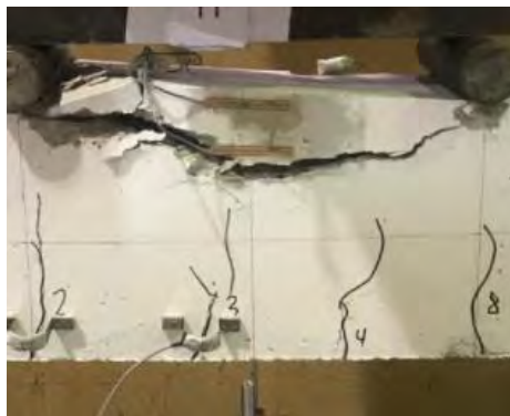
Figure 61: Failure mode of beam 2G20UR.
