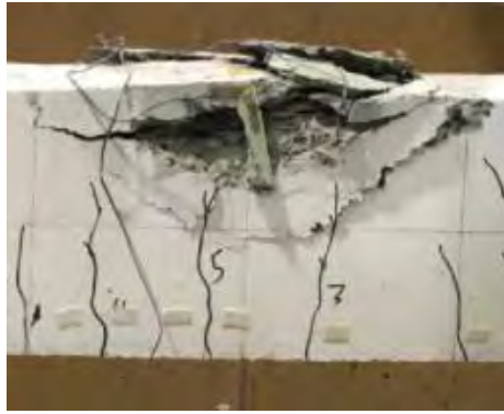
Figure 59 : Failure mode of beam 2G26ER.
