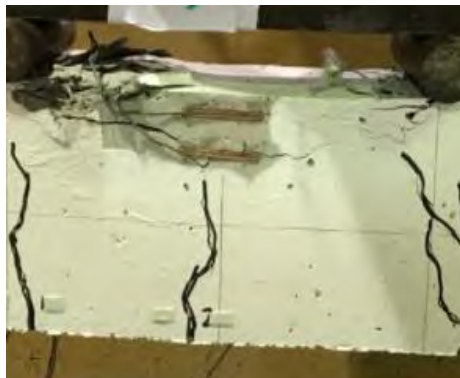
Figure 73: Failure mode of beam 2S12.
