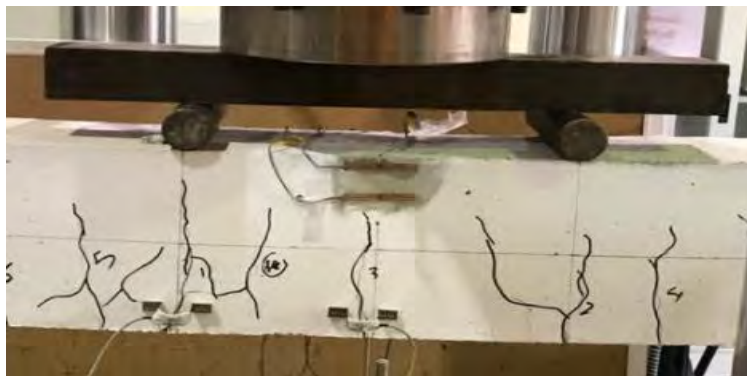
Figure 79: Cracks propagation of beam 2G10UC.
