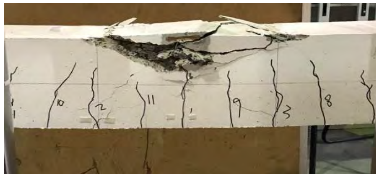
Figure 76: Cracks propagation of beam 3G16EC.
