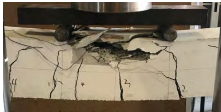
Figure 87: Cracks propagation of beam 2B10EC.
