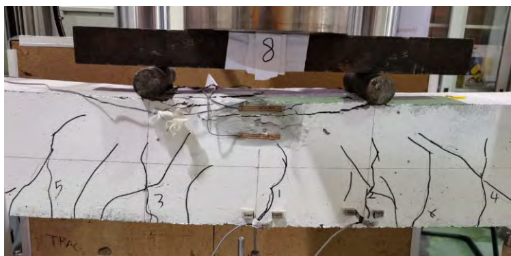
Figure 81: Cracks propagation of beam 2G20ER.
