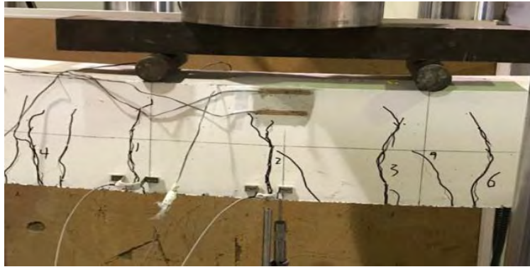
Figure 78: Cracks propagation of beam 2G8UC.
