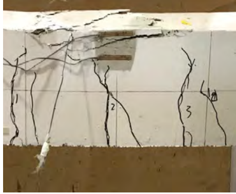
Figure 55: Failure mode of beam 2G8UC.
