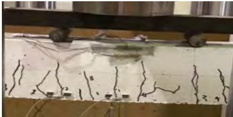
Figure 91: Cracks propagation of beam 3B16EC.
