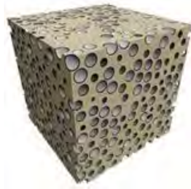
Figure 2: Closed-cell syntactic foams [14]
