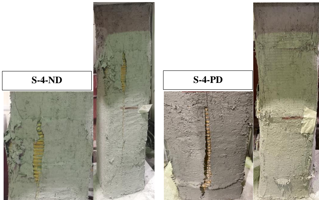
Figure 32: Group A failure modes.
