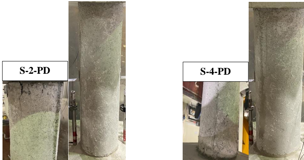
Figure 18: Pre-damaged columns after unloading.
