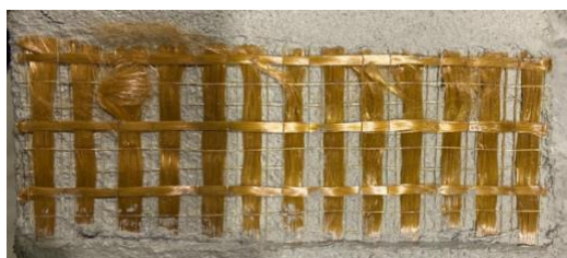
Figure 17: Sample of PBO-FRCM provided by RureGold.
