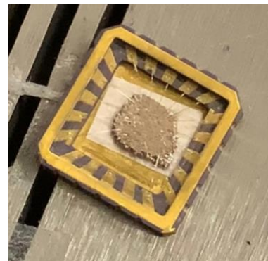
Figure 16: Fe_xCu_{100-x} after soldering wires onto it to load into the Cryogen System
