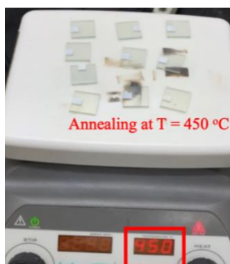
Figure 22: Annealing of TiO 2 at 450°C
