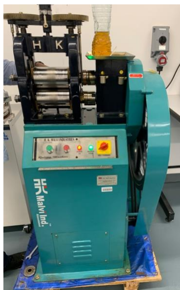
Figure 19: Flattening the Al-FeCu electrode using the HK Malvi Wire Sheet Roller
