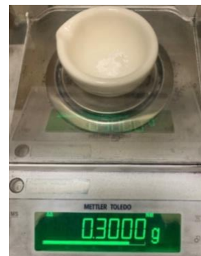
Figure 21: Addition of PEG to the TiO 2
