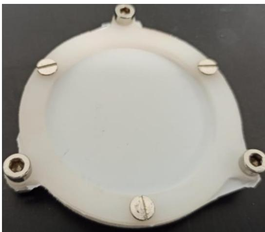
Figure 3-4: The membrane sheet fixed between Teflon hoops
