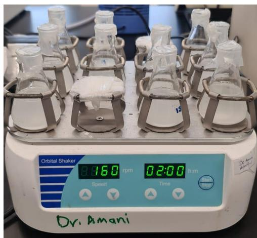
Figure 3-2: Batch adsorption experiment
