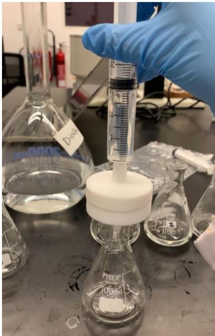
Figure 3-5: Membrane filtration setup
