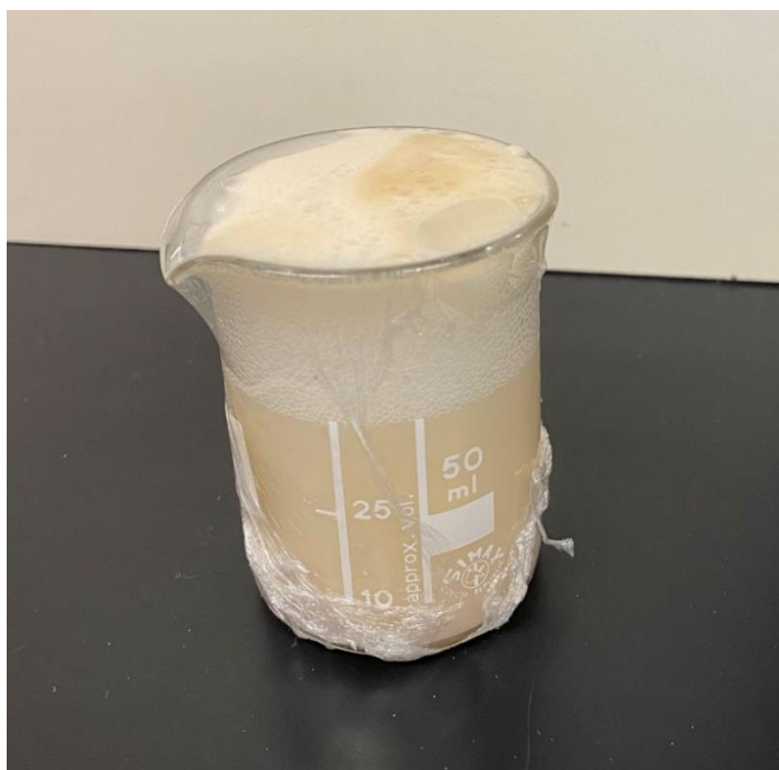
Figure 4-4: Created sludge layer on top of solution as representation of proper yeast activation.
