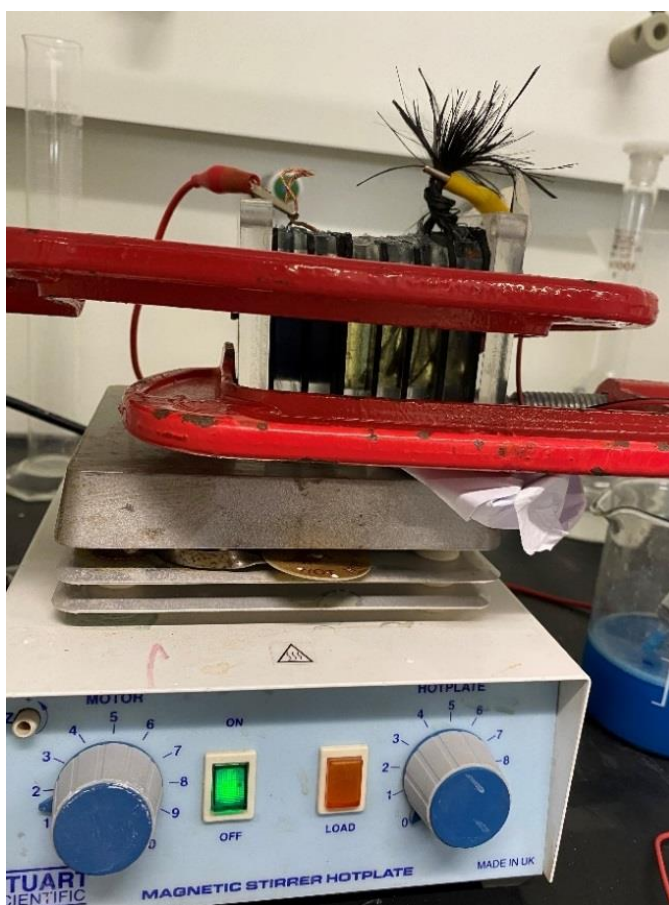
Figure 4-1: Schematic of the cubic dual chamber of MFC.
