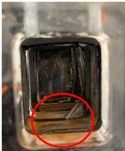
Figure 5-15: Precipitation of the Au(III) ions as Au(OH)_3 at the bottom of cathode chamber.
