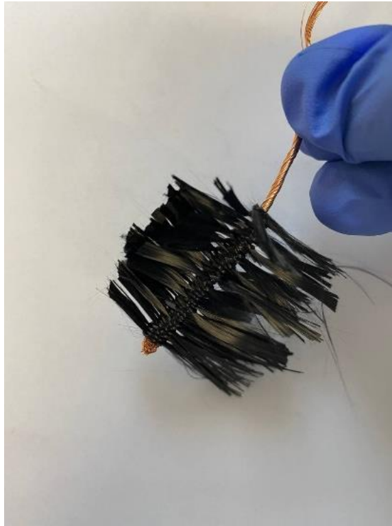
Figure 4-2: Carbon brush as electrode for the anode chamber
