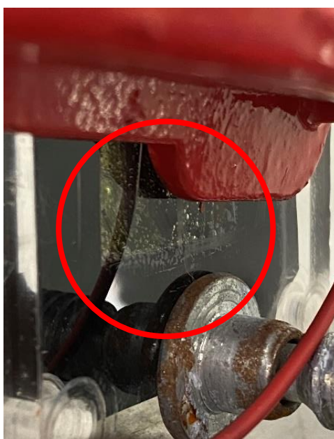
Figure 5-3: Bubble creation in the cathode compartment during the performance of the cell.
