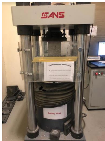
Figure 23: Concrete crushing setup.
