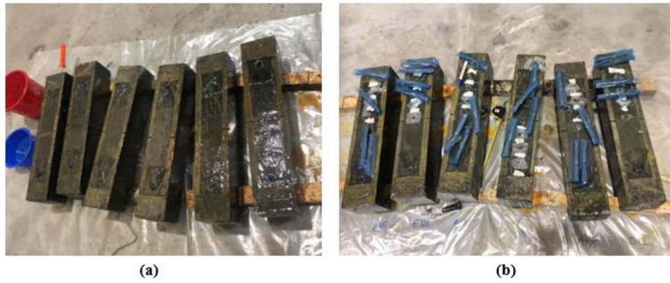
Figure 33: After strengthening: (a) dry prisms; (b) dry prisms with strain gauges.
