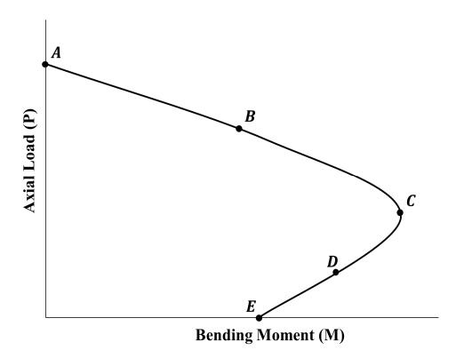
Figure 3. A typical axial load-bending moment interaction diagram with its significant control points.
