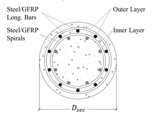
Figure 1. Concrete column's cross-section with double-layer reinforcement.
