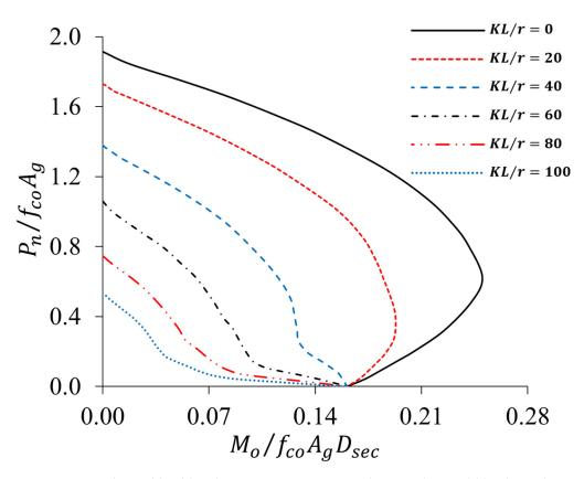
**Figure 4.** A sample axial load-bending moment interaction diagram that could be derived using provided data (group G6, strength level 2,  $\rho_l = 4\%$ ).
