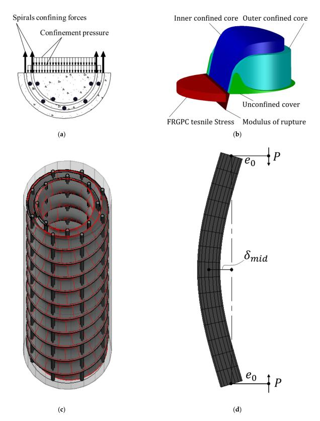
**Figure 2.** Modeling considerations: (**a**) confinement pressure change through cross-section layers, (**b**) stress-strain distribution along the cross-section, (**c**) the effectively confined cores of the inner and outer reinforcing layers, and (**d**) a buckled column with additional moment at its mid-height cross-section.
