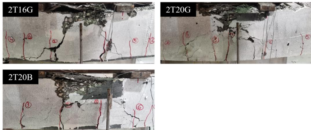
Figure 4-3: Failure modes and cracking patterns of over-reinforced beams.
