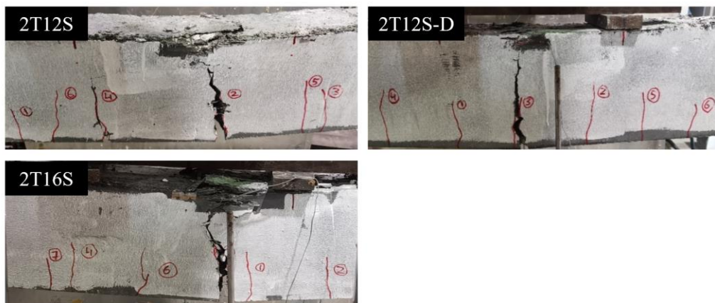
Figure 4-2: Failure modes and cracking patterns of steel reinforced beams.
