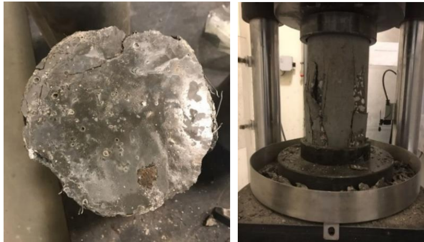
Figure 3-10: Cylinders after testing.
