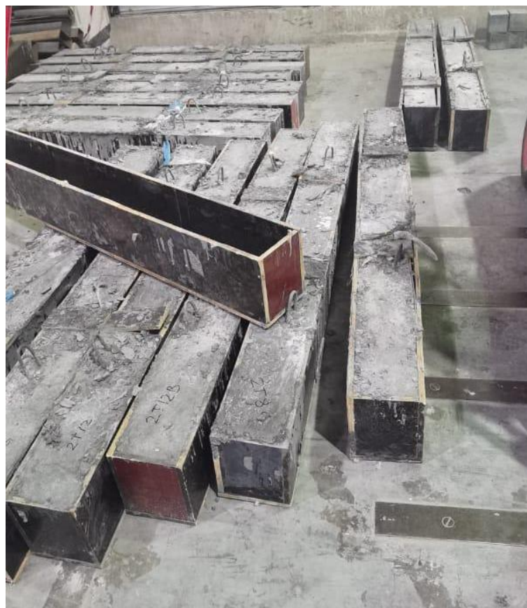
Figure 3-14: Casting process of specimens.
