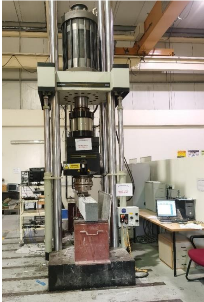
Figure 3-17: Universal Testing Machine (UTM).
