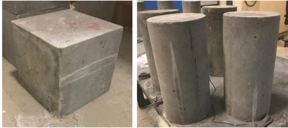
Figure 3-9: Cubes and cylinders before testing.
