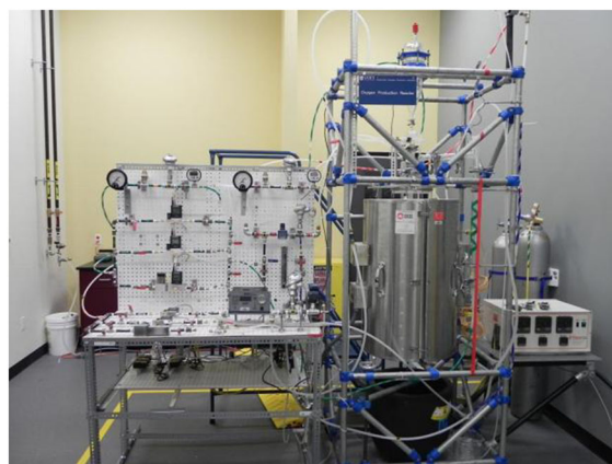
Figure 6. High-temperature experimental unit for copper oxychloride decomposition and oxygen production.
