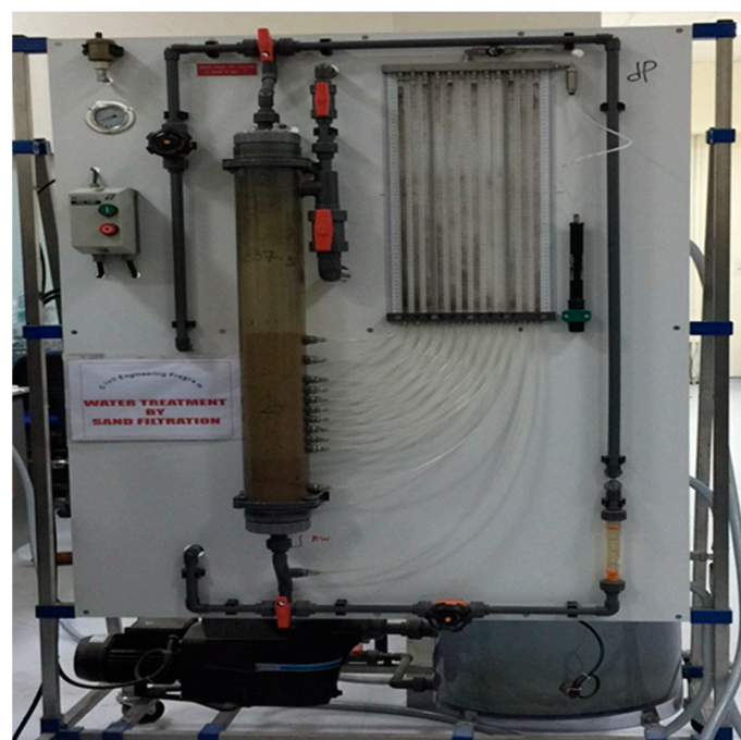
Figure 2. Sand filtration experimental setup.
