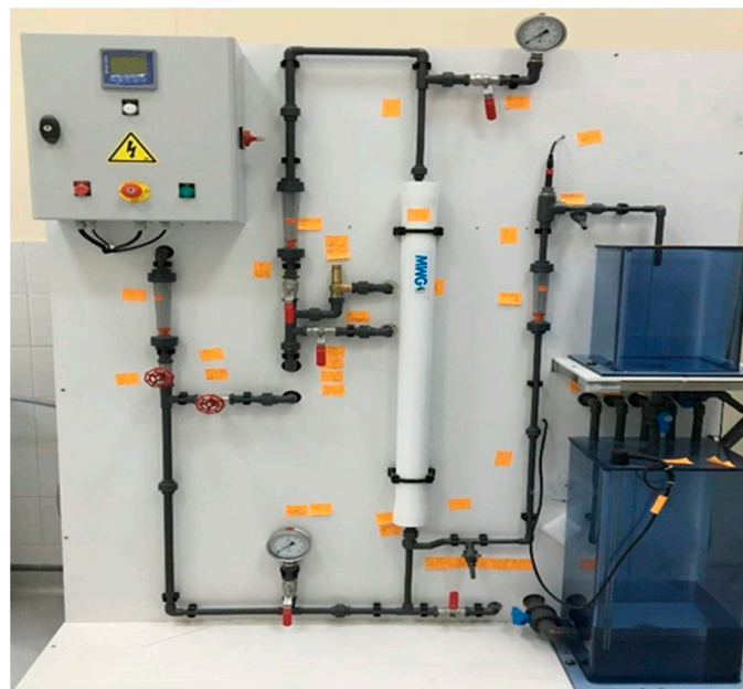
Figure 1. Simplified membrane experimental setup.
