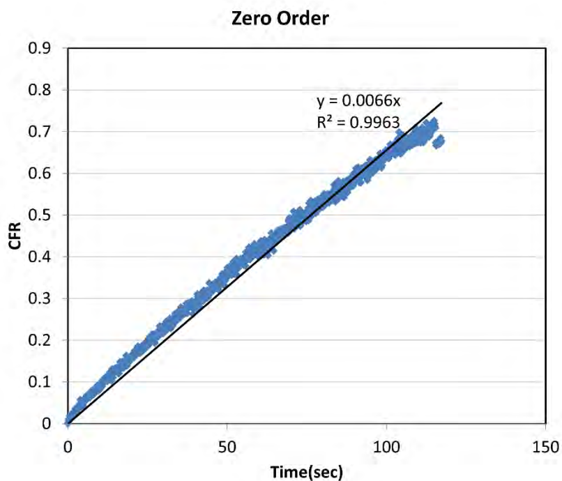
Figure B-1 Calcein release from B-2 Calcein release from eLiposomes (Batch 1) at 6.2 mW/cm 2 fitting Zero-order Model
