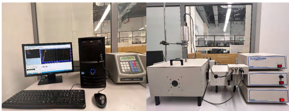
Figure 3-3 Low-frequency ultrasound probe and phosphorescence spectrofluorometer setup for drug release
