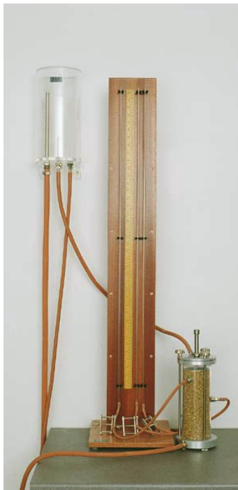
FIGURE 3.11 Constant Head Permeability Cell and Apparatus [37]
