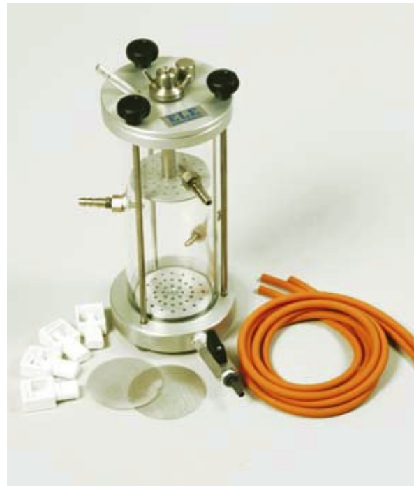
FIGURE 3.11 Constant Head Permeability Cell and Apparatus [37]
