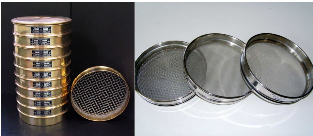
FIGURE 3.1 Sieve used for a gradation and size test [34]
