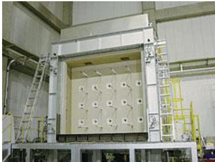
(a) Structural Fire Testing Furnace (Large scale, for Walls) at the Center for Fire Science and Technology in Tokyo, Japan
