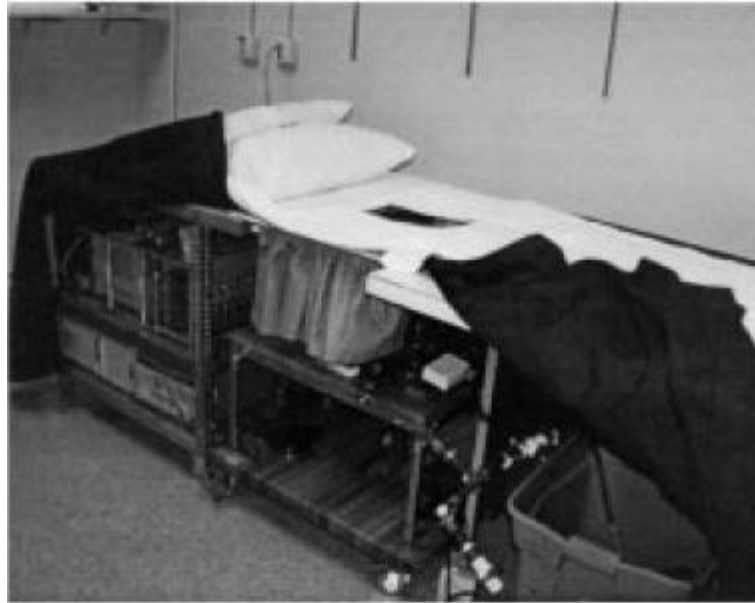
Figure 2.13 The clinical prototype for active microwave imaging of the breast developed by Meaney et al.[18]
