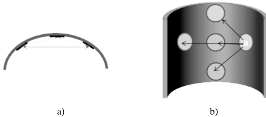
Figure 3.5 Crosstalk between retina elements in a cylindrical retina a) top view, b) front view
