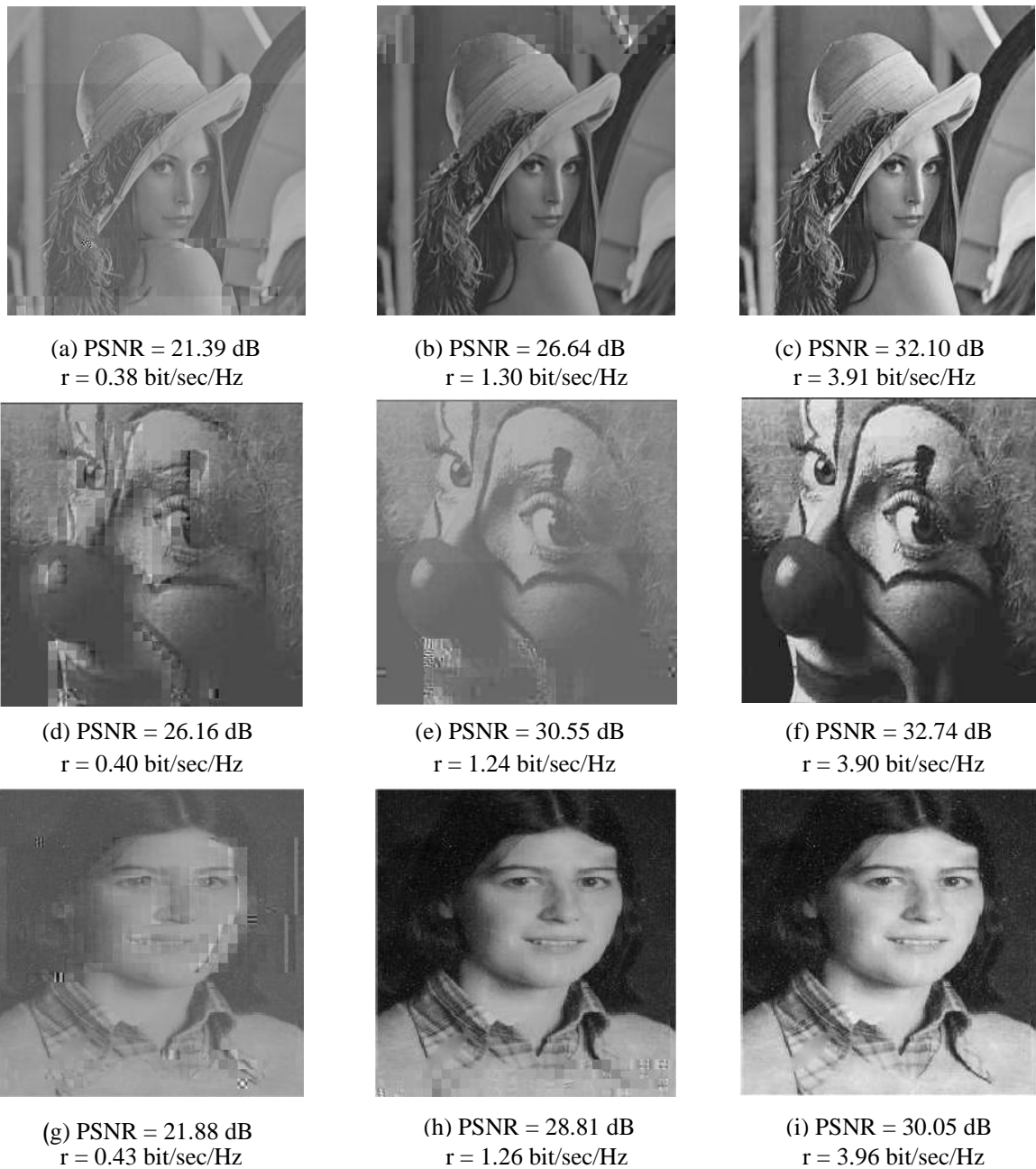
Figure 4.8: Transmitted images over Rayleigh fading channel using adaptive modulation and channel coding scheme.
