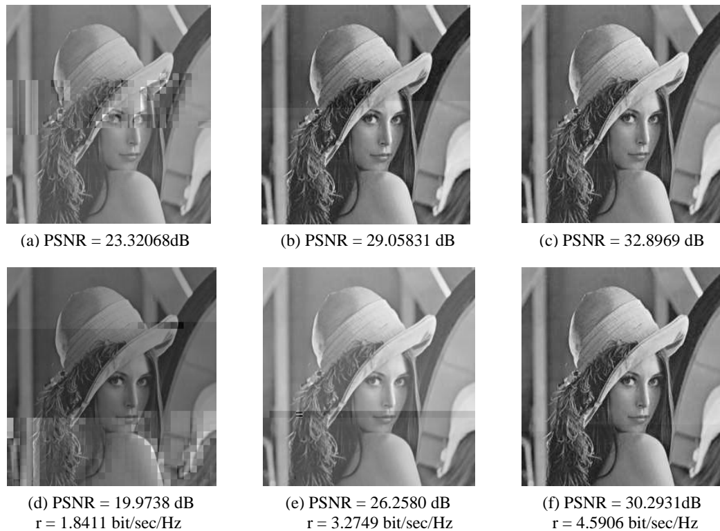
Figure 4.3: Transmitted Lena image over Rayleigh fading channel using adaptive scheme.
