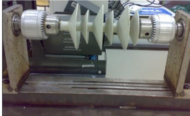
Figure 2-3: Mechanical Setup including: Drill heads, Ball Bearing, Stand
