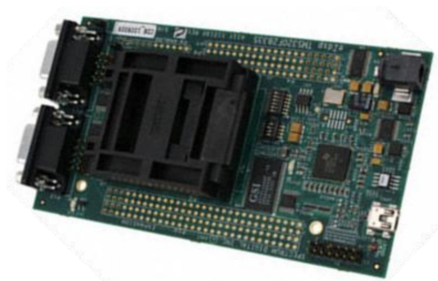
Figure 6.1: Texas Instrument's TMS320F28335 DSP board
