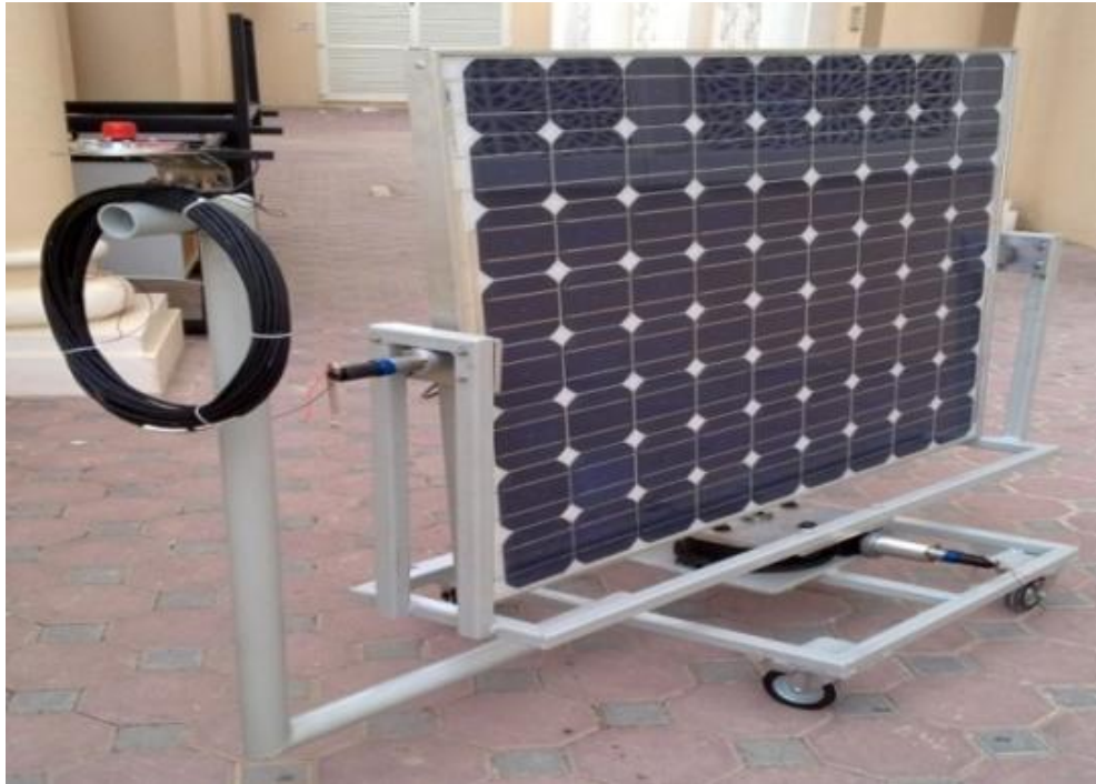
Figure 6.2: Front view of the solar tracker mechanism (panel in vertical position)
