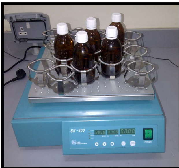
Figure 3.1: Samples on Shaker Table
