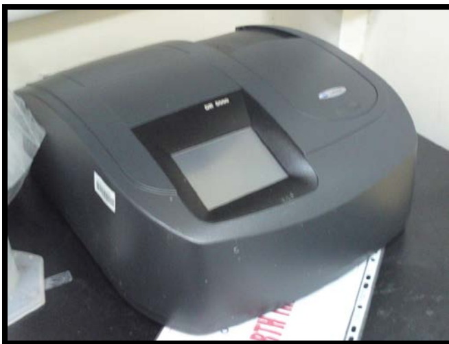
Figure 3.4: HACH DR 5000 Spectrophotometer
