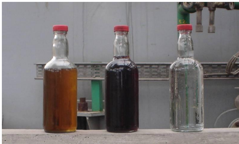
Figure 1.2: Two Refinery Spent Caustic Samples (left and center) and Treated Effluent (right) [18]
