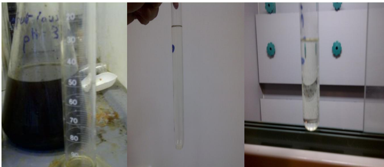
Figure 2.12: Refinery Spent Caustic (left) and Two Treated Samples (middle and right)
