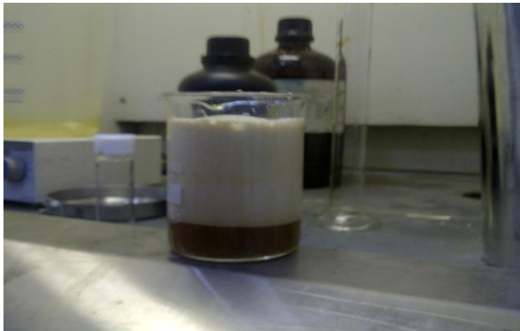
Figure 2.3: Foaming in Fenton's Reaction after Few Seconds
