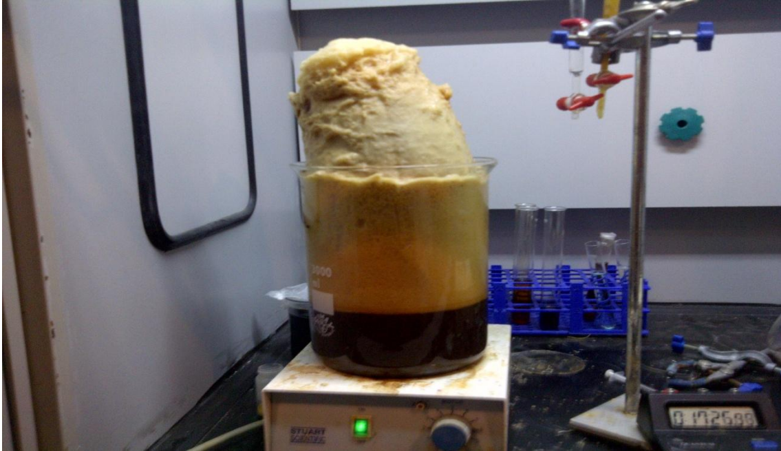
Figure 3.2: Foaming During Scale Up
