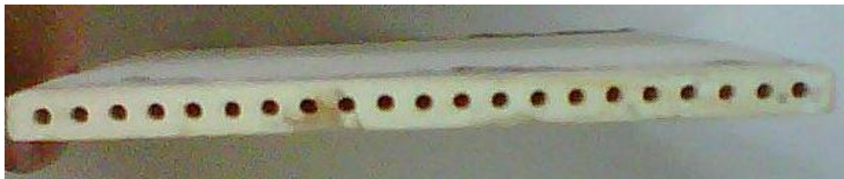
Figure 34: Holes at the side of the ceramic support for the flow of feed solution
