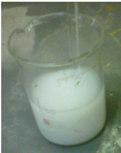
Figure 29: Reaction of magnesium sulfate with barium hydroxide to produce magnesium hydroxide and barium sulfate precipitates.
