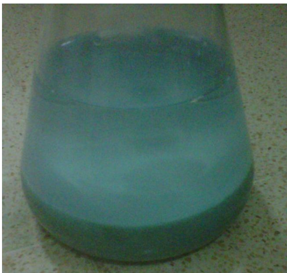
Figure 40: Formation of copper hydroxide and barium sulfate precipitate mixture
