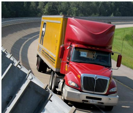
Figure 5: Front drag-reducing device.[8]
