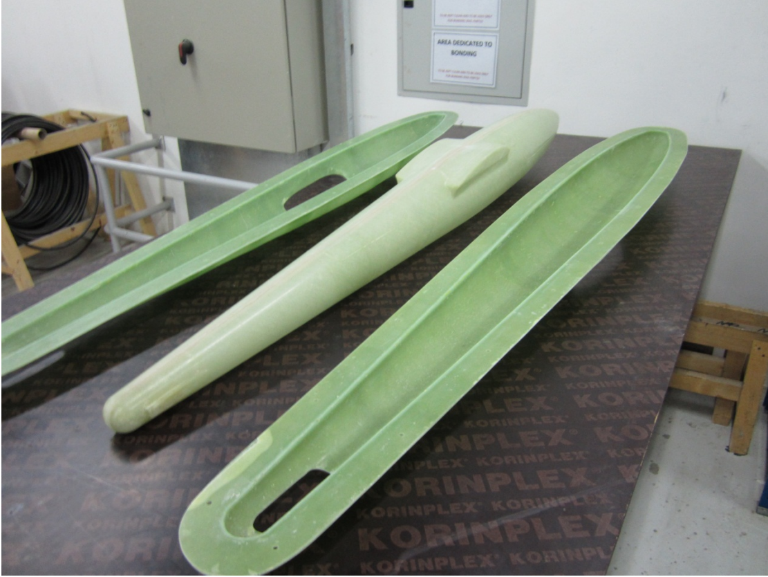
Figure 55 Fuselage Final Product Sample and The Assembly Jigs
