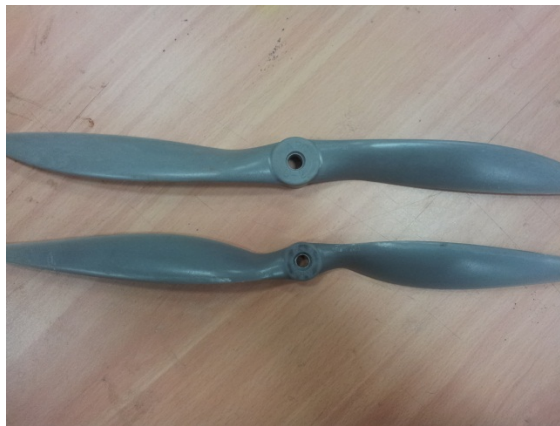
Figure 49 Electric Propeller at the bottom and Combustion Engine Propeller at the top
