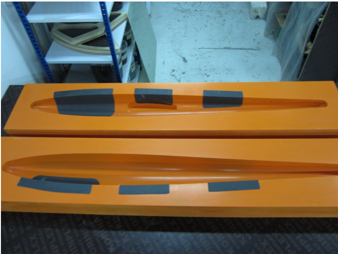
Figure 53 The Mold for Fuselage Part Built by Premier Composite
