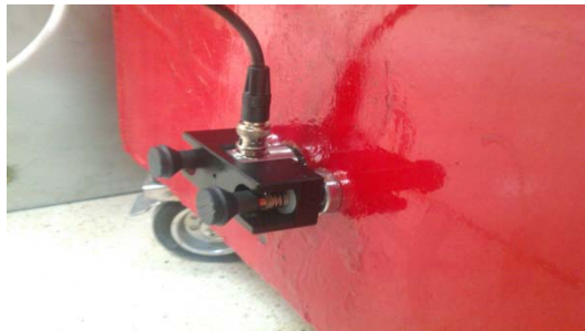
Figure 9: AE sensor installation
