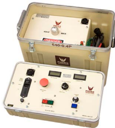
Figure 16: High voltage source and the control panel
