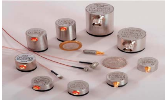
Figure 8: Different types and sizes of AE sensors [26]
