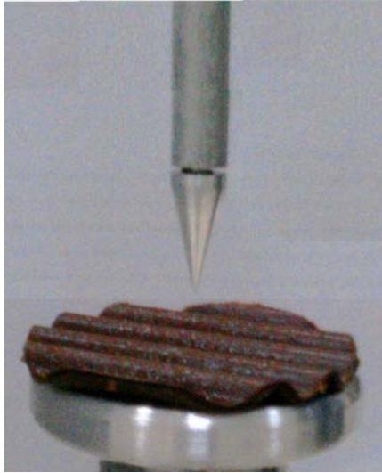
Figure 20: Surface discharge electrode
