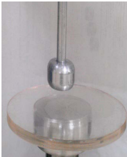
Figure 21: Void discharge electrode
