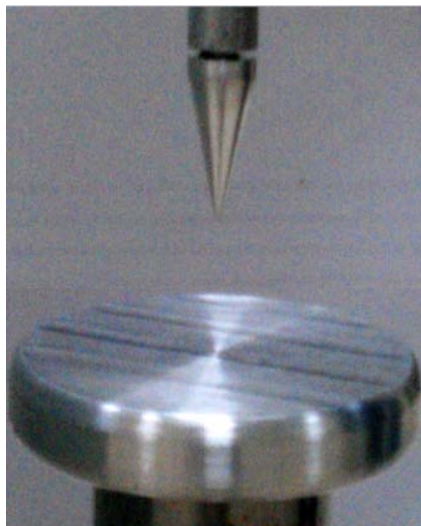
Figure 18: Sharp point to ground electrode
