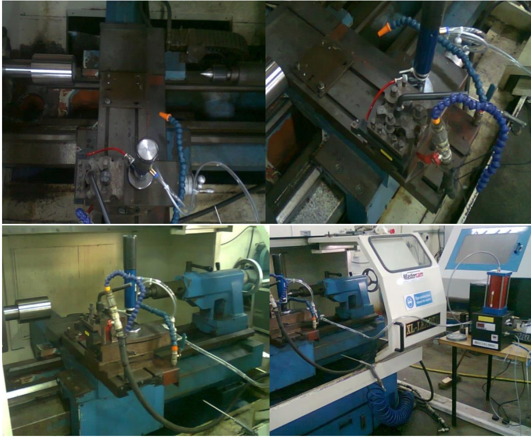
Fig. 16 Eco-Lubric Booster system.
