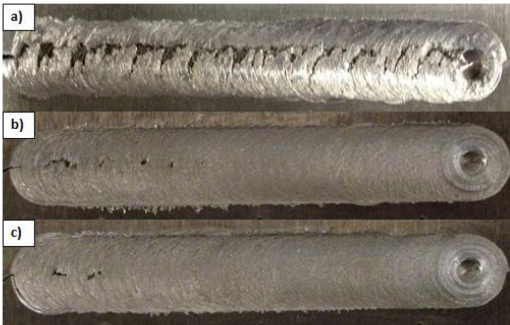
Figure 4.1 – In air FSW samples at 75 mm/min and (a) 800 rpm, (b) 1000 rpm and (c) 1200 rpm
