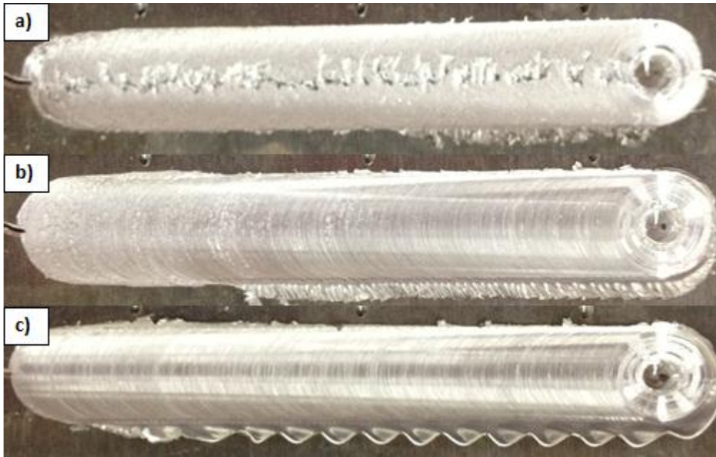
Figure 4.1 – In air FSW samples at 75 mm/min and (a) 800 rpm, (b) 1000 rpm and (c) 1200 rpm
