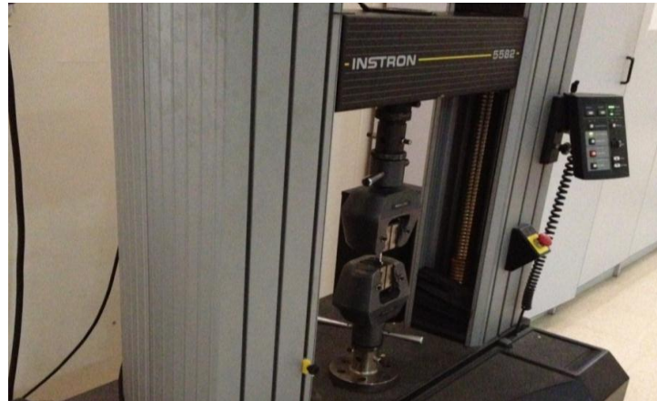
Figure 3.5 - Instron machine used for tensile testing
