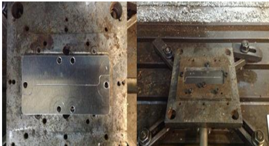
Figure 3.1 - Close up view of sample prior to welding and holding fixture
