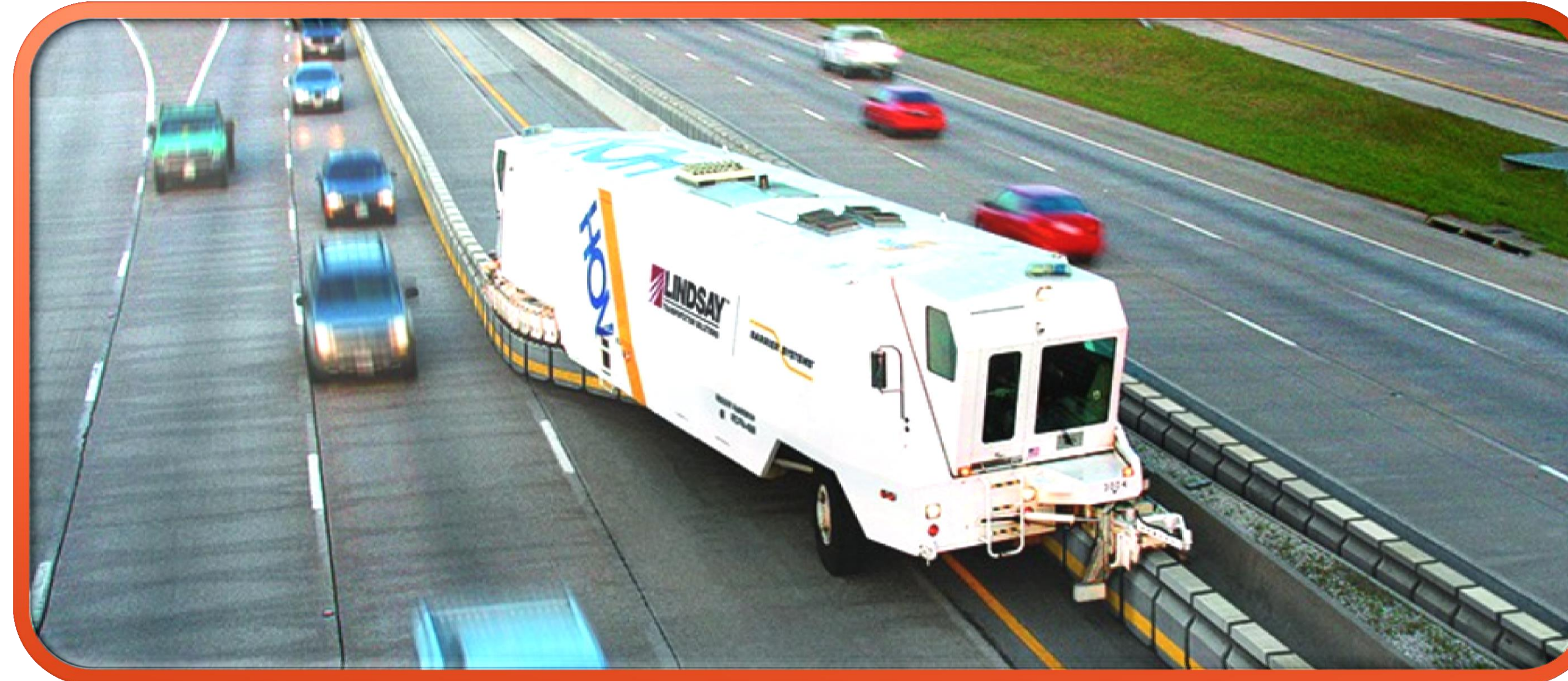
Figure 2: A zipper machine adjusting the lane [3]
